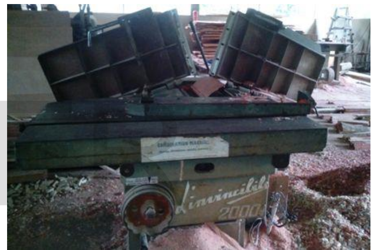
Plate 5: Combination machine used for conversion of wood samples into dimensions
